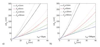
Fig. 7 Average (solid lines) and maximum (dotted lines) ohmic potential drop in the solution for Design A with a TCO as a function of electrode length,  $l_{\rm el}$ , for different electrolyte heights,  $h_{\rm e}$ , and for  $t_{\rm sep}=10~\mu{\rm m}$  (a) and 500  $\mu{\rm m}$  (b).
