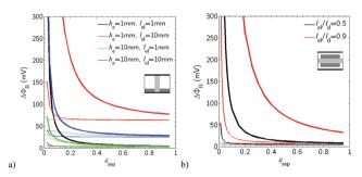
**Fig. 13** Average ohmic potential drop,  $\Delta \Phi_{\rm R}$  (solid line), and average ohmic potential drop minus the average potential drop over the separator,  $\Delta \Phi_{\rm R} - \Delta \Phi_{\rm R,sep}$  (dotted line), as a function of separator porosity for  $t_{\rm sep} = 10~\mu{\rm m}$  (thin lines) and  $t_{\rm sep} = 500~\mu{\rm m}$  (thick lines), for various dimensions of Design A (a) and Design B at  $h_{\rm e} = 1~{\rm mm}$  and  $t_{\rm el} = 1~{\rm mm}$  (b).
