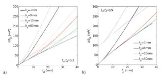
**Fig. 8** Average ohmic potential drop in the solution for Design B with a TCO with (a)  $l_{\rm el}/l_{\rm d}=0.5$  and (b)  $l_{\rm el}/l_{\rm d}=0.9$  as a function of the electrode length,  $l_{\rm el}$ , for various electrolyte heights,  $h_{\rm e}$ , and for  $t_{\rm sep}=10~\mu{\rm m}$  (solid line) and  $t_{\rm sep}=500~\mu{\rm m}$  (dotted line).
