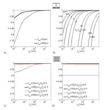
Fig. 11 Hydrogen collection yield, due to diffusion, of Design A (a and b) and Design B (c and d), for boundary condition option (i): the opposite electrode surface is at zero concentration (a and c) and option (ii): the opposite chamber is at zero concentration (b and d), for various component dimensions.
