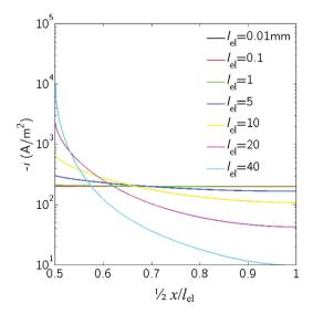
**Fig. 4** Current density distribution along the catalyst layer of the cathode for Design A (separator starts at  $x/l_{\rm el}/2=0.5$ ) with TCO,  $h_{\rm e}=1$  mm,  $t_{\rm sep}=10$  µm, and for cathode lengths 0.01 mm <  $l_{\rm el}<40$  mm.
