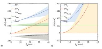
Fig. 5 Average (lines) and variation along the electrode (bands around lines) for the total device overpotential  $(\Delta \Phi_s)$ , ohmic losses  $(\Delta \Phi_R)$ , potential losses over separator only  $(\Delta \Phi_{R,sep})$ , and anode/cathode reaction overpotentials  $(\eta_{op,a/c})$  with TCO (a) and without TCO (b) as a function of  $l_{el}$ , for Design A at  $h_e = 1$  mm and  $t_{sep} = 10$  µm.
