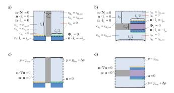
**Fig. 2** Computational domain and boundary conditions of Design A (a and c) and Design B (b and d) for species and charge conservation (a and b), and mass and momentum conservation (c and d). Concentration boundary conditions (green, red, blue) which account for operational condition options (i) to (iii) are described in the text.
