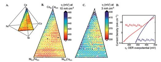
Fig. 2 Analysis of a pseudoternary section of the  $(Ni-Fe-Co-Ce)O_x$  catalyst space. (A) A planar slice through the tetrahedron of Fig. 1B that intersects the composition regions of interest. The pseudoternary map of the planar slice showing the overpotential (B) at 10 mA cm<sup>-2</sup> as in Fig. 1 and (C) at 3 mA cm<sup>-2</sup> from CV data. (D) The catalytic current extracted from CV measurements is shown for the representative high-Ce and low-Ce catalysts.
