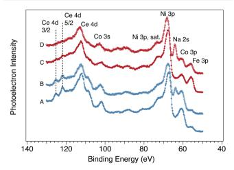
Fig. 4 High-resolution XPS spectra of the Ce4d, Ni3p, Co3p, and Fe3p region from the GC RDE samples. (A) High-Ce composition ascalcined at 350 °C and (B) after 2 h CP at 10 mA cm $^{-2}$ . (C) Low-Ce composition as-calcined at 350 °C and (D) after 2 h CP at 10 mA cm $^{-2}$ . The Na 2s peak only appears on samples exposed to 1.0 M NaOH during electrochemical testing.
