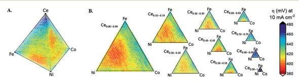
Fig. 1 Performance map of  $(Ni-Fe-Co-Ce)O_x$  oxygen evolution catalysts. The composition map of the overpotential required for performing oxygen evolution at 10 mA cm<sup>-2</sup> from CP measurements is shown (A) in the quaternary composition tetrahedron and (B) as a series of pseudoternary slices through the quaternary space.
