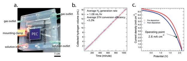
Fig. 2 (a) Photograph of an integrated, membrane-free solar-driven water-splitting device. (b) Rate of production of hydrogen gas in the cathode compartment. The average rate of  $H_2$  production was calculated to be 1.08 mL  $h^{-1}$  from a linear fit of the experimental data. (c) Currentvoltage characteristic of the triple-junction a-Si:H cell before and after catalyst deposition. The operating current density of the integrated device, 2.6 mA cm<sup>-2</sup>, is indicated by a green circle.
