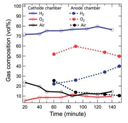
Fig. 4 Time evolution of the gas composition (H<sub>2</sub>, O<sub>2</sub> and air) in the cathode compartment (solid lines) and the anode compartment (dashed lines).
