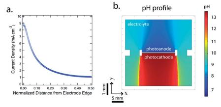
Fig. 3 (a) Current density as a function of the normalized distance from the photoelectrode edge from the simulation, (b) cross-sectional pH profiles in the membrane-free device from the COMSOL Multiphysics simulation
