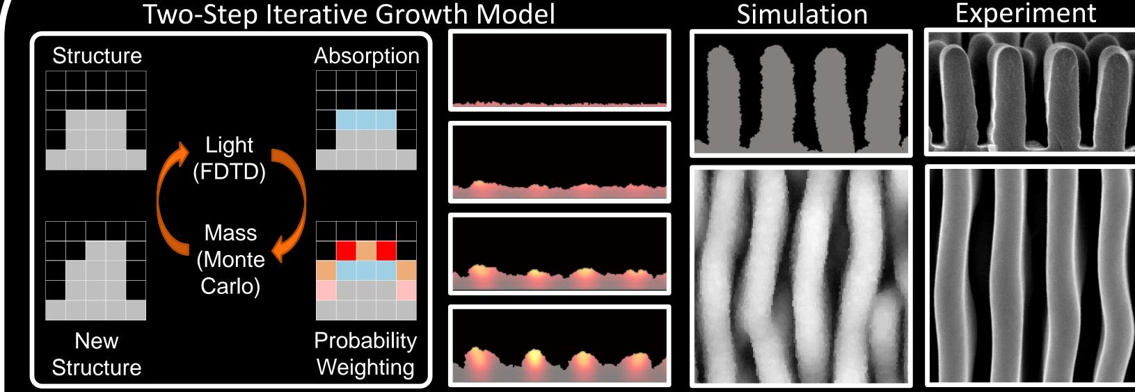
Simulations using iterative model: FDTD method first utilized to calculate light absorption profile. Then, a Monte Carlo method used to add mass preferentially to high absorption areas. No empirical inputs beyond the material complex refractive index. Experimental agreement suggests morphologies are fully optically determined.
