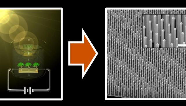
In analogy to natural phototropism, utilize unstructured illumination and capitalize on inherent anisotropies in light-material interactions to optically instruct growth of complex mesostructures in three-dimensions without a template nor photomask.
