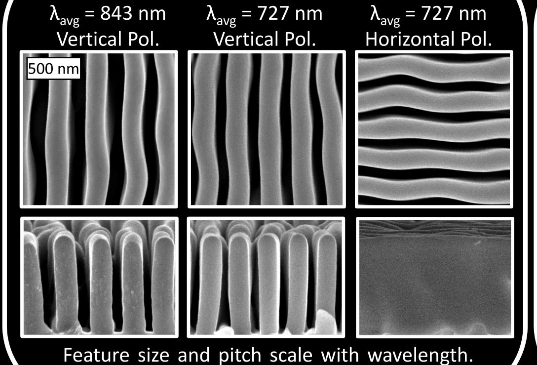
Polarization sets in-plane orientation.
