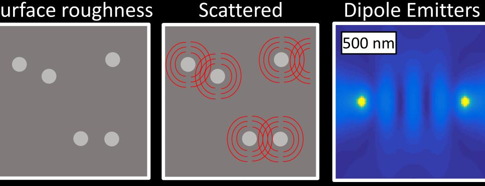
Initial film nuclei scatter the incident illumination. This optical interaction was modeled using two dipole emitter sources: interference fringes were observed between the sources. This spatiallyoscillating light intensity profile effects spatiallyanisotropic rates of photoelectrochemical growth.
